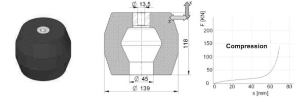
Recommended deformation constant on the X axis (max mm.): 28
