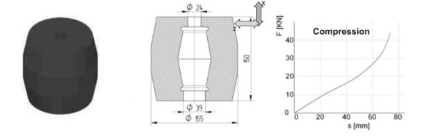
Recommended deformation constant on the X axis (max mm.): 40
