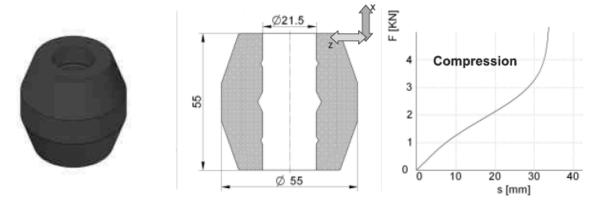
Recommended deformation constant on the X axis (max mm.): 15
