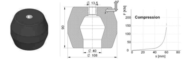
Recommended deformation constant on the X axis (max mm.): 23
