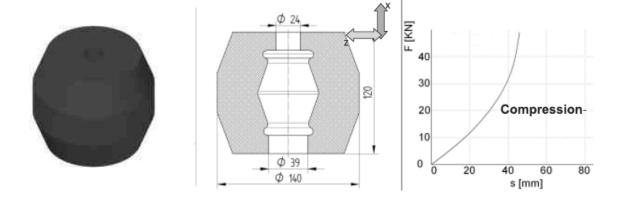
Recommended deformation constant on the X axis (max mm.): 30
